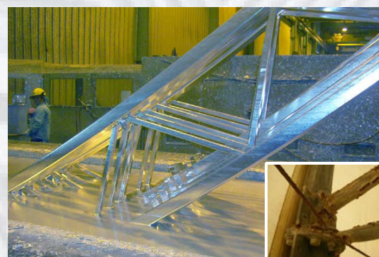
Galvanizing Steel in Zinc Bath
